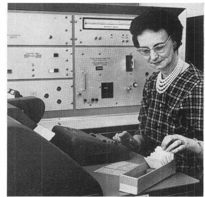
NEW FILM DENSITOMETER, operated by Rita Hodgden (3311-2), measures the X or gamma radiation exposure to the film within the new badges. This information is automatically punched on IBM cards as employees' lifetime radiation exposure records.
